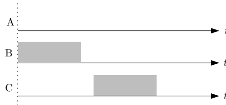
Figure 18.17 Session activity. Grey areas indicate the time when a session is transmitting a frame. Note the transmissions of B and C do not overlap in time.
